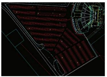
Note: Always keeping in mind the type of data I want to extract. For example, if I need a point for a tree, it doesn't have to be as precise, but if it's a building corner or manhole, in that case, the process needs to be optimized and carefully verified. This project also included the property boundary, which was captured using RTK with an OPUS solution via PPK
