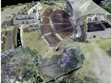
Note: As you can see in the images, there are areas of the structure's roof that are not covered, as we focused more on the lower levels, knowing we have that data from the drones. In a case where we needed to cover the roof, we would move my setups differently and most likely use the spider tripod, which has a 15' extension. It has its particularities in terms of use, but that could be covered in another article.
