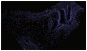
After verifying and modifying the triangle interpolation, we generated the contour lines from my final surface.
